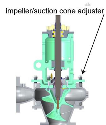
*Note: Depending on the pump model, one full turn of the adjuster is equal to 0.063" - 0.072". Turning the adjuster one "flat" or one "point" is equal to about 0.010" - 0.012". In the screw pumps this changes the impeller to cone gap by about .004".*
